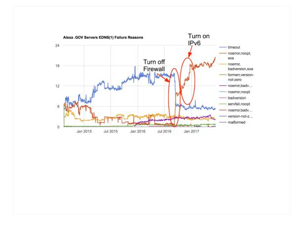
The step changes in the blue timeout line and the red no OPT record line show a large DNS hoster turning off the firewall in front of the DNS servers exposing the mishandling of EDNS queries by them. They then enabled IPv6 on those servers which is visible in the four step jumps as each region in turn was on.
