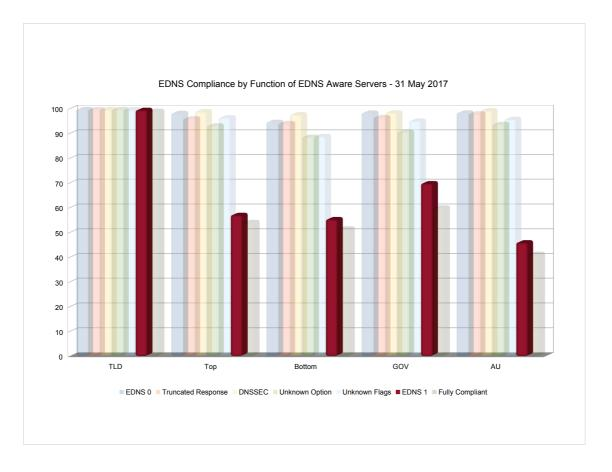
The red columns are servers that correctly answered EDNS(1) queries. Queries with unsupported EDNS versions are supposed to be responded to with rcode BADVERS and the version field set to the highest EDNS version supported by the server.
