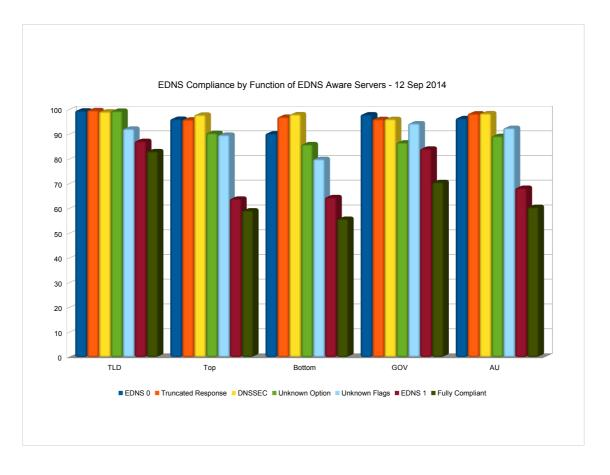
When we started we found was that DNSSEC was reasonably well supported but that unknown EDNS options and unknown EDNS flags were not well supported, and that unknown EDNS versions were very poorly supported. This was despite RFC specifying how to handle unknown EDNS options and unknown EDNS versions.
